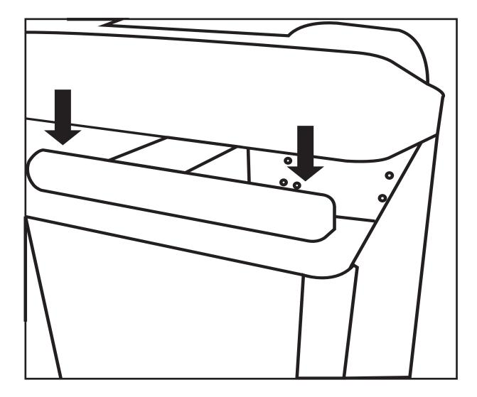
Place trash bag over bag holder sides shown within the dotted lines. Do not let trash bag drape outside bin over graphic display panels. Bag Size Required: 17"W x 44"L
