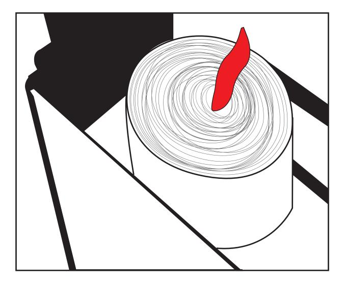
Feed towel/wipe through Adjustable Tension Regulator hole opening then adjust tension.
